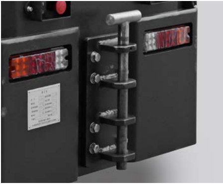
Reinforced traction couplers with three adjustable heights ensure reliable connection to various trailers.
