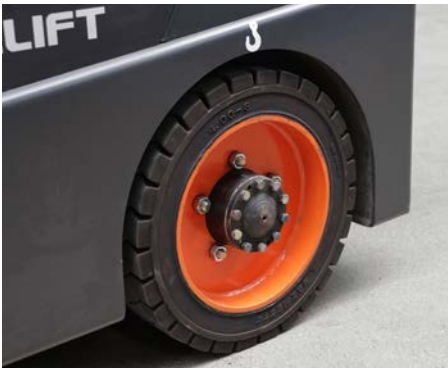
Equipped with solid rubber tires. Lifting points clearly marked for transporting vehicle.
