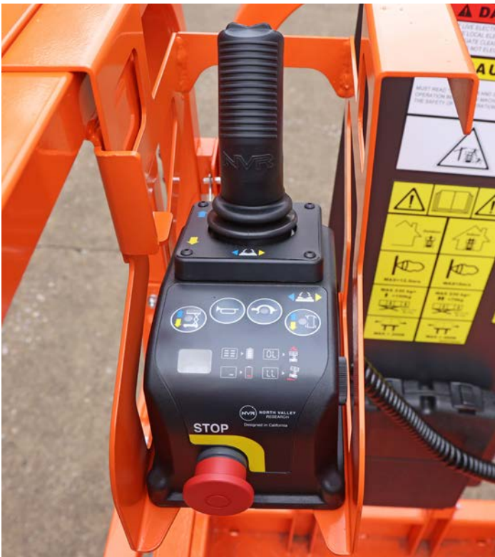
Proportional control handle for lifting and traveling ensures smooth operation.
