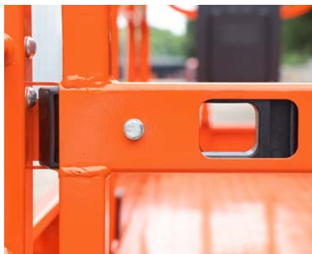
Self-locking platform door for operator safety.
