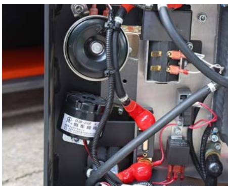
Horn and motion buzzer serve as motion alarms.
