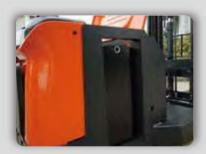
Standard side battery extraction, with battery rollers. Battery replacement efficient and safe for multiple shift operations and ease of maintenance.
