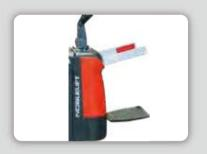
Integrated foldable ride-on platform with protective arms, power steering, internal chassis design allows short overall length, and tightest turning radius in industry.
