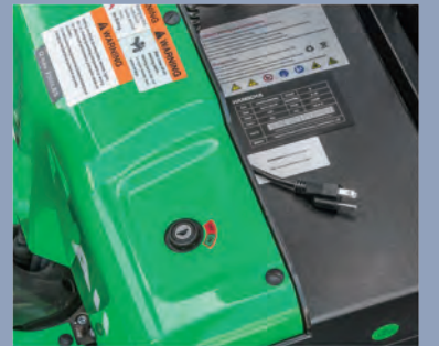
Features a built-in charger and a maintenance free battery.
