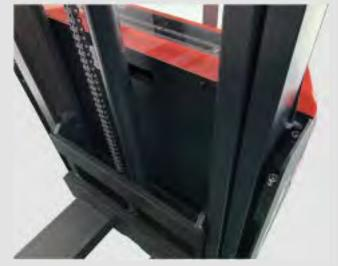
Support legs are made out of solid steel (not tube) to have enough rigidity to ensure the
