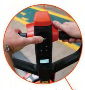
The ability to operate the unit with the tiller in the upright position allows working in confined spaces.
