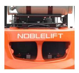
Angled exit ports direct engine air away from the operator and the cab to help operators stay cool.
