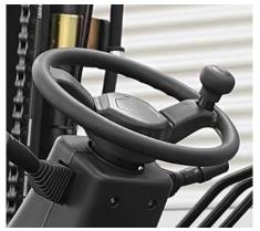
On-Demand Fully Hydrostatic Power Steering (FHPS) guarantees smooth steering, preventing over-run and kickback. Spinner knob allows easier one-handed steering.
