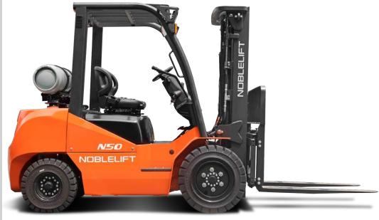
Modular frame is designed based on the same chassis as the NOBLELIFT Diesel and Electric forklifts. Main components and configurations are the same. Spare parts inventory is minimized to reduce service and maintenance costs.
