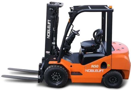
Modular frame is designed based on the same chassis as the NOBLELIFT LPG and Electric forklifts. Main components and configurations are the same. Spare parts inventory is minimized to reduce service and maintenance costs.
