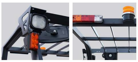
Equipped with LED lamps: LED rear work lights, headlights, strobe and safety blue light. Bright light with low power consumption provides excellent visibility.
