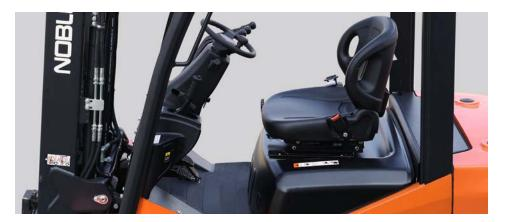
The large, ergonomic cab and user-friendly design ensures operator comfort throughout the entire work shift. Low entrance height provides operator easy and safe access. Deluxe suspension, fully adjustable seat reduces vibration to the driver to effectively reduce driver fatigue for all sizes of operators.
