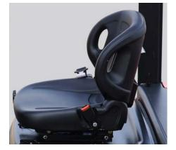
Operator Presence System (OPS) — When operator is not in seat, the hydraulic lift and tilt controls automatically lock out and traveling is disabled.
