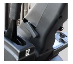
The angle of the steering column is easily adjusted with a lever on the left-hand side of the steering column.
